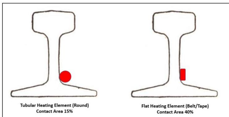
Figure 3 Illustration of Contact Areas of Heating Elements with the Rail Web
