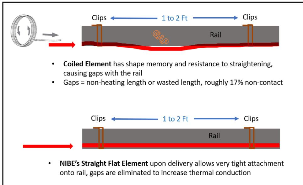
Figure 8 Demonstration of Element Attachment Gap and Its Elimination
