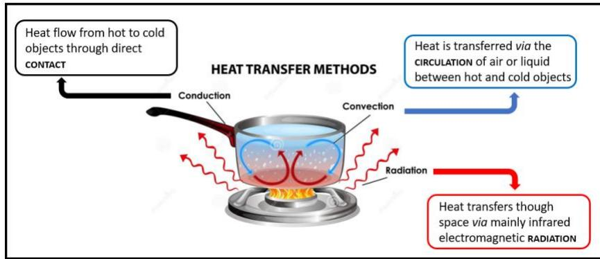
Figure 7 Demonstrations of Heat Transfer
