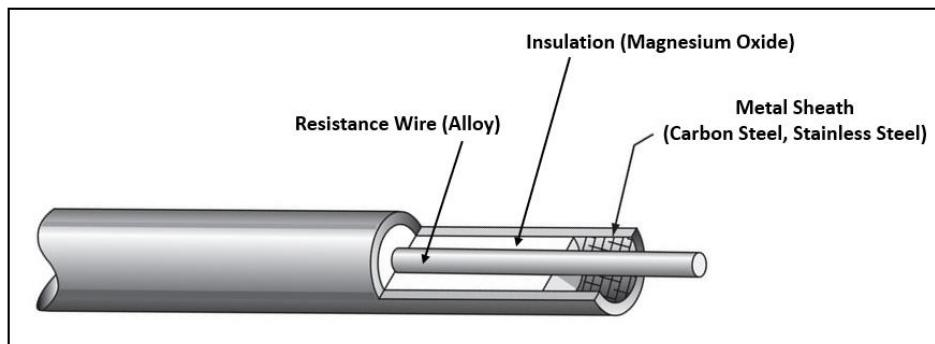
Figure 2 Illustration of a Tubular Heating Element
