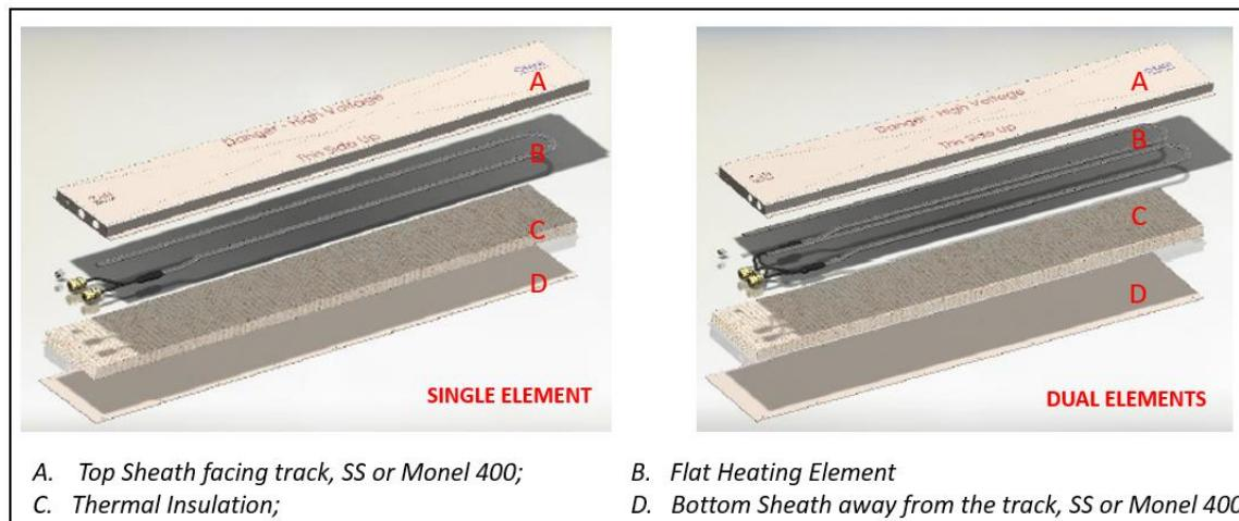
Figure 6 Examples of PAN Heaters
