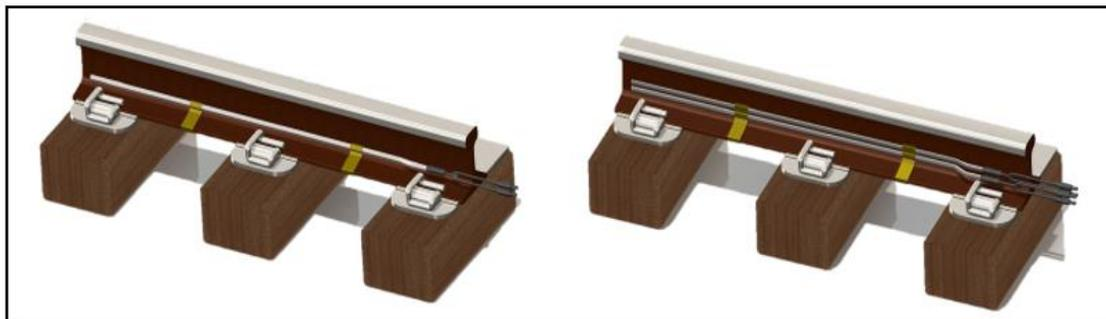
Figure 5 Flat Heating Element Installed on the Rail
