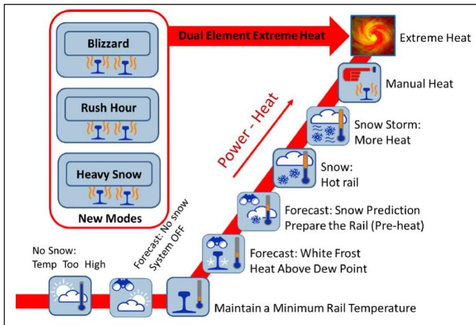
Figure 11 The Power of Heating Is Regulated Based on Weather Conditions
