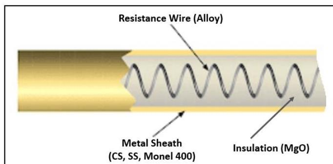
Figure 10 Demonstration of a Tubular Heating Element with Helical Resistance Wire.
